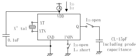
Note: The AC characteristics are observed using an oscilloscope on pin Q.
