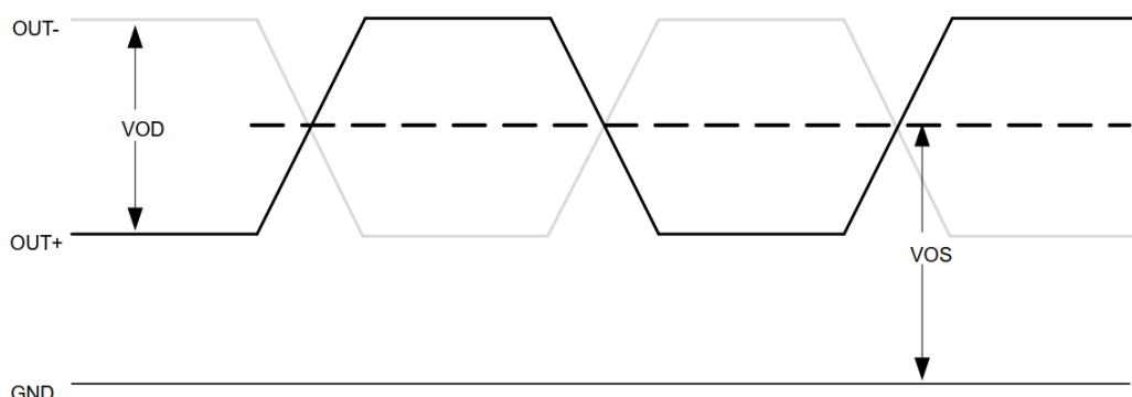
Figure 4: LVDS Voltage Levels per Differential Pin (OUT+/OUT-)
