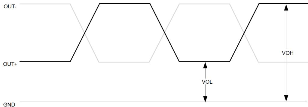
Figure 2: LVPECL Voltage Levels per Differential Pin (OUT+/OUT-)
