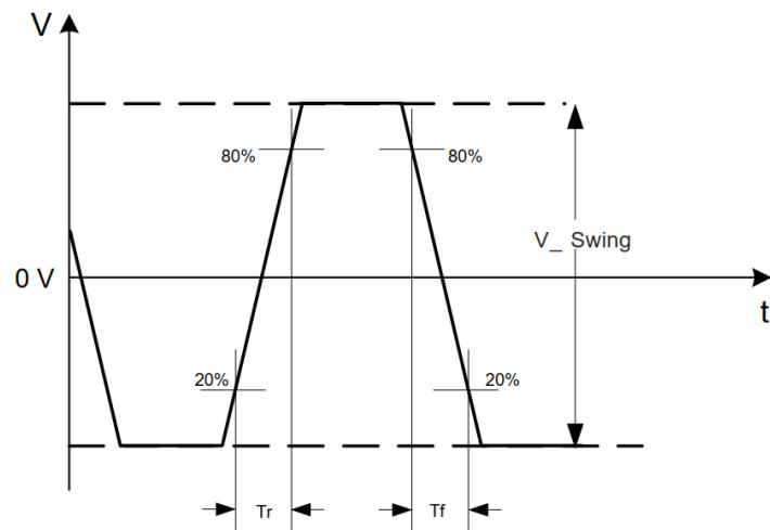
Figure 3: LVPECL Voltage Levels across Differential Pair
