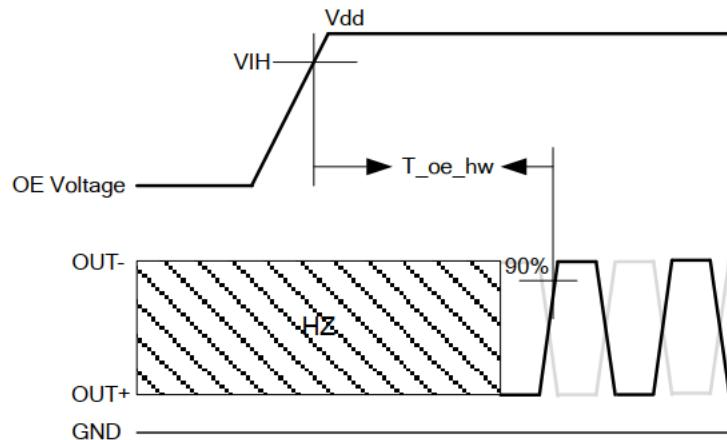
Figure 6: Hardware OE Enable Timing
