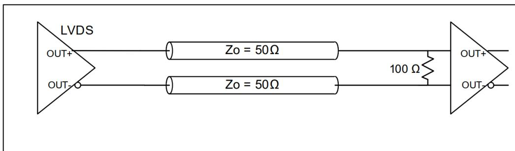
Figure 12: LVDS single DC termination at the load
