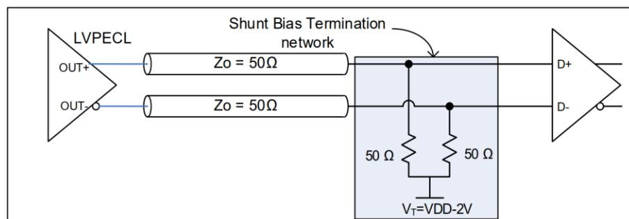
Figure 11: LVPECL with DC-coupled parallel shunt load termination
