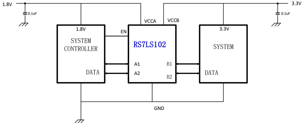
**Figure 10 Application Circuit**
