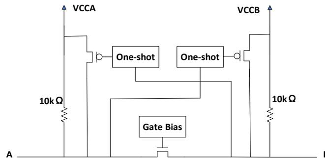
**Figure 8 Level Shifter Architecture**
