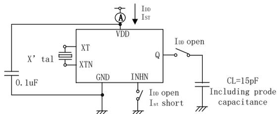
Note: The AC characteristics are observed using an oscilloscope on pin Q
