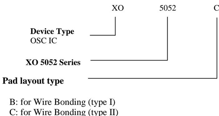
The XO5052xy series are miniature crystal oscillator module ICs. The oscillator circuit stage has constant current drive, significantly reducing current consumption and crystal current, compared with existing devices, and significantly reducing the oscillator characteristics supply voltage dependency.
