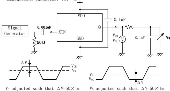
XTN input signal: 1Vp-p, sine wave
