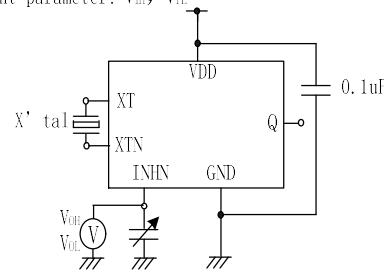
$V_{IH}$ : Voltage is 0V to  $V_{DD}$  transition that changes the output state.
