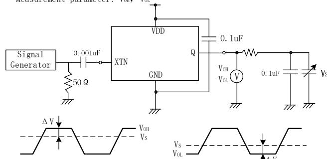
$V_s$  adjusted such that  $\Delta V=50 \times I_{DD}$
