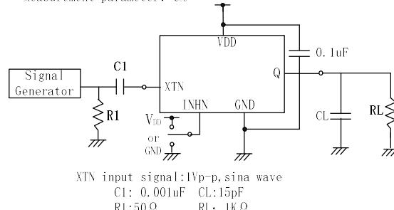
XTN input signal: 1Vp-p, sine wave
