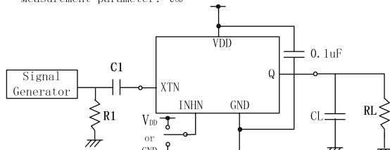
XTN input signal: 1Vp-p, sine wave
