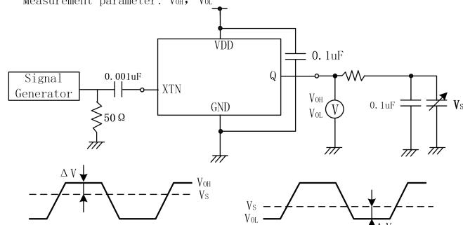
XTN input signal: 1Vp-p, sine wave
