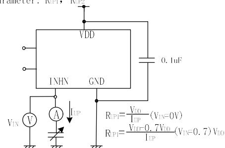
$$R_{P1} = \frac{V_{DD}}{I_{UP}} \quad (V_{IN}=0V)$$
